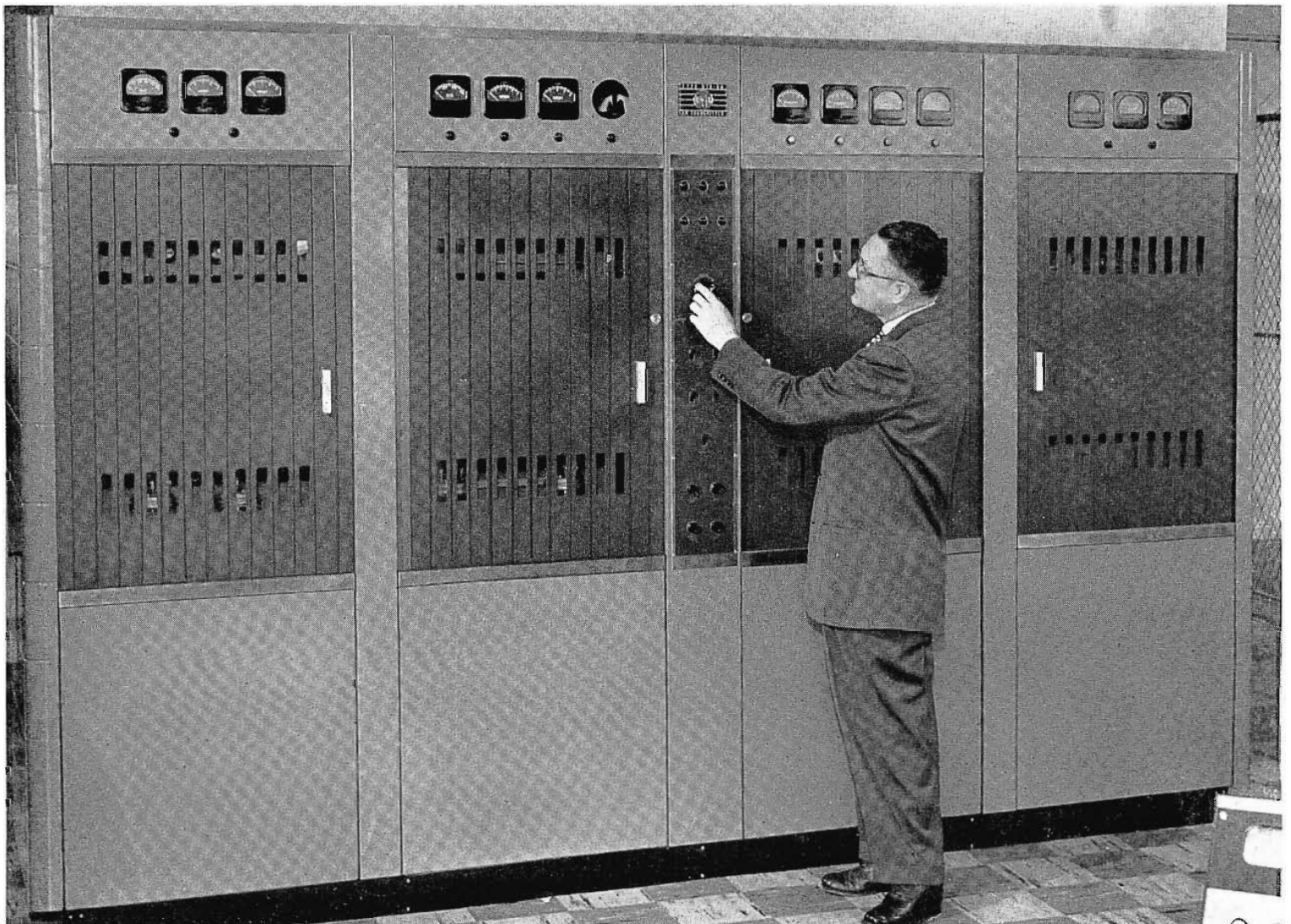
WTMJ William H. Hebal, Chief Engineer of AM, adjusting the power-output control. A manually operated selsyn motor, used as a phase-shifter, provides front-panel control of the output plate voltage. ▼
