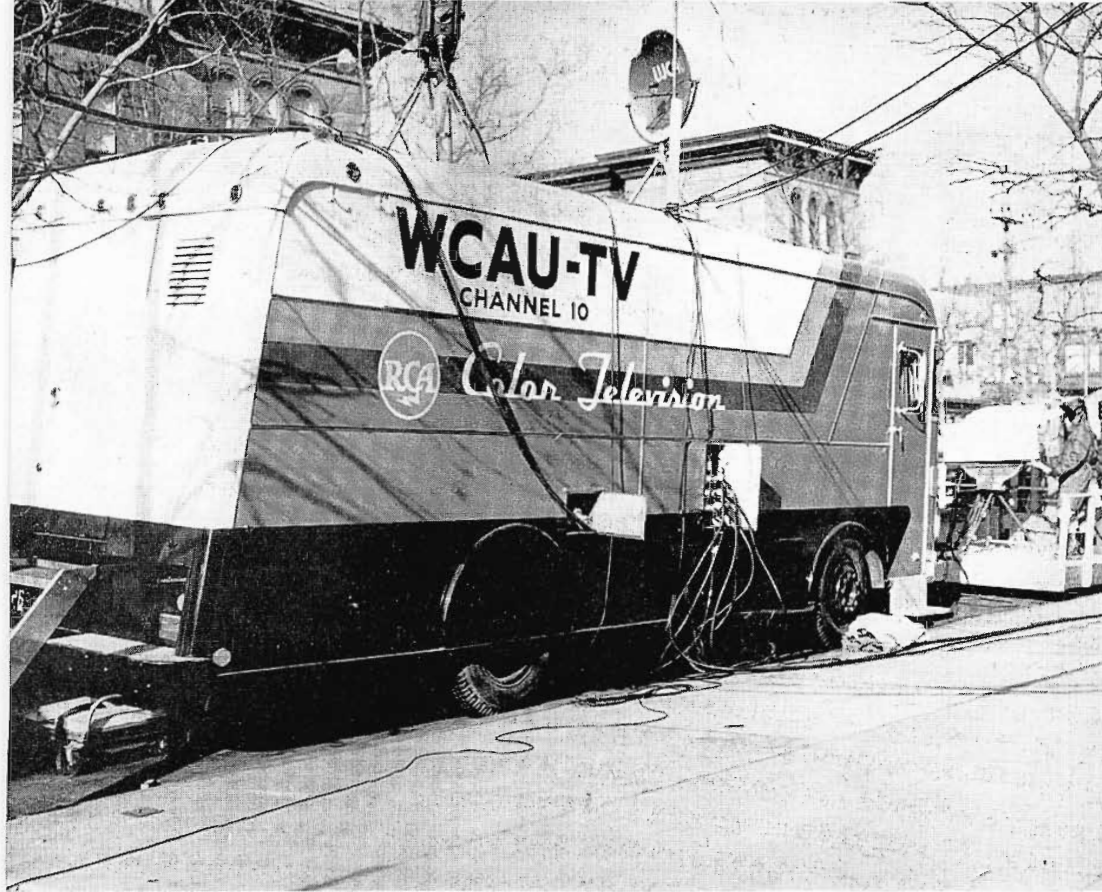
FIG. 5. On this side of the color mobile unit, the receptacle at the right contains sockets for connecting audio, video, telco lines and microwave facilities. At the left is the power-line receptacle.
