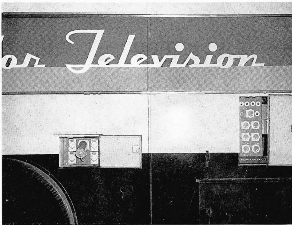
FIG. 12. Curb-side of truck showing power and audio/video terminal receptacles—power input on left—audio/video on right.
