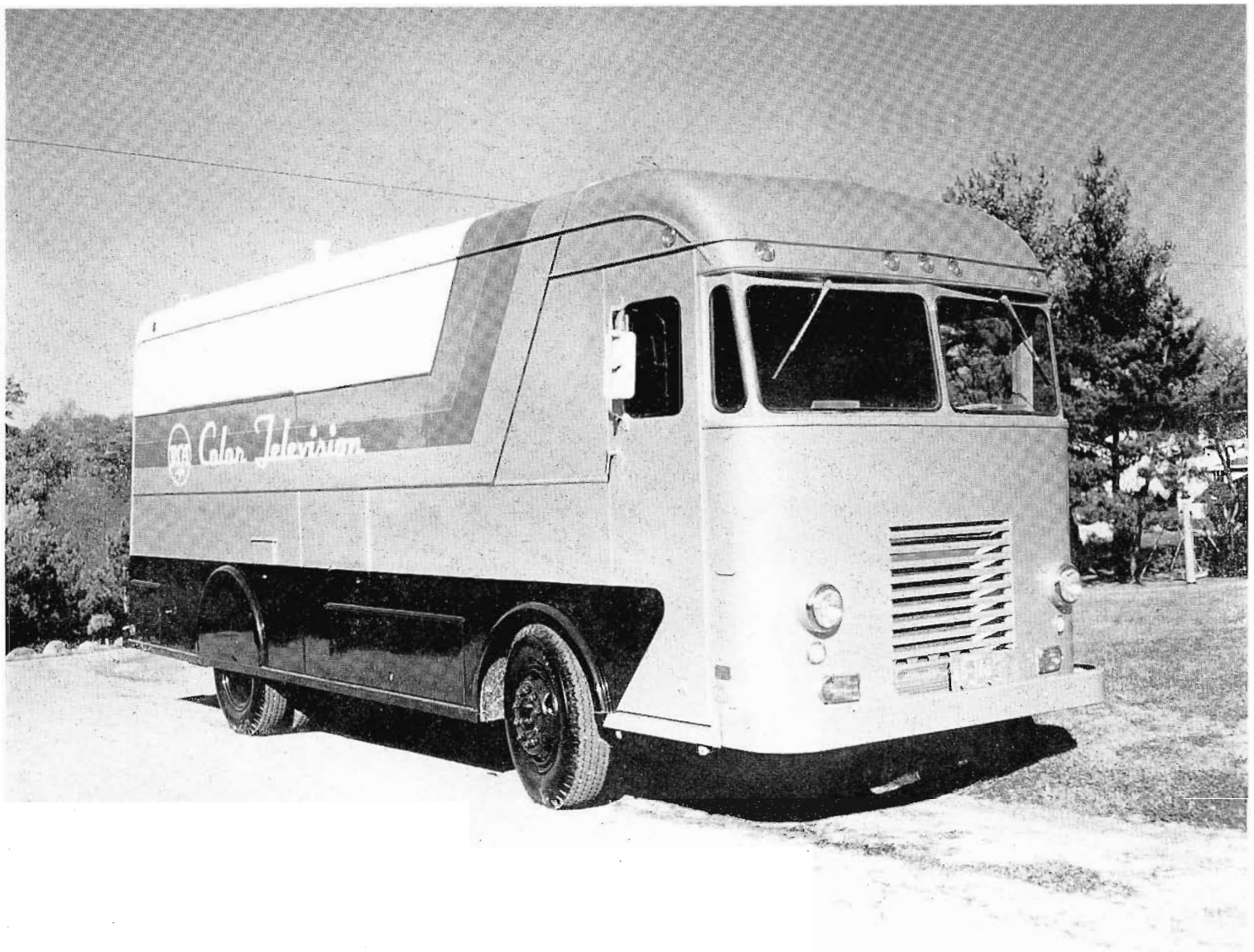
FIG. 1. External view of RCA Color Television Mobile Unit—designed to house two live color camera chains and associated equipment.
